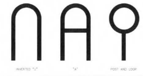
Figure 4.6.9(D)(12) - 1, Typical Type I Bicycle Racks
